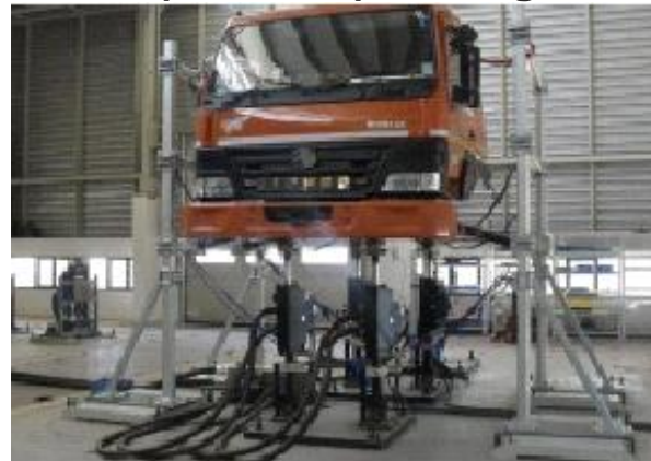
Cabin (5 Poster) test rig
