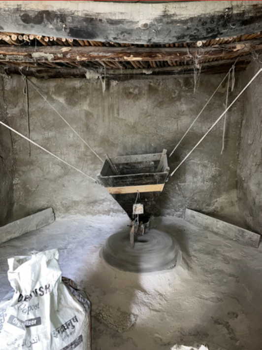
Water-powered grain mill, Aranu. A traditional mechanism still in use today.
