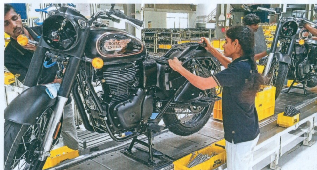
(Main picture) The 349cc, J-series engine is being assembled by a woman technician has 265 parts. (Below) A new Bullet motorcycle nearing completion is inspected on the assembly line.
