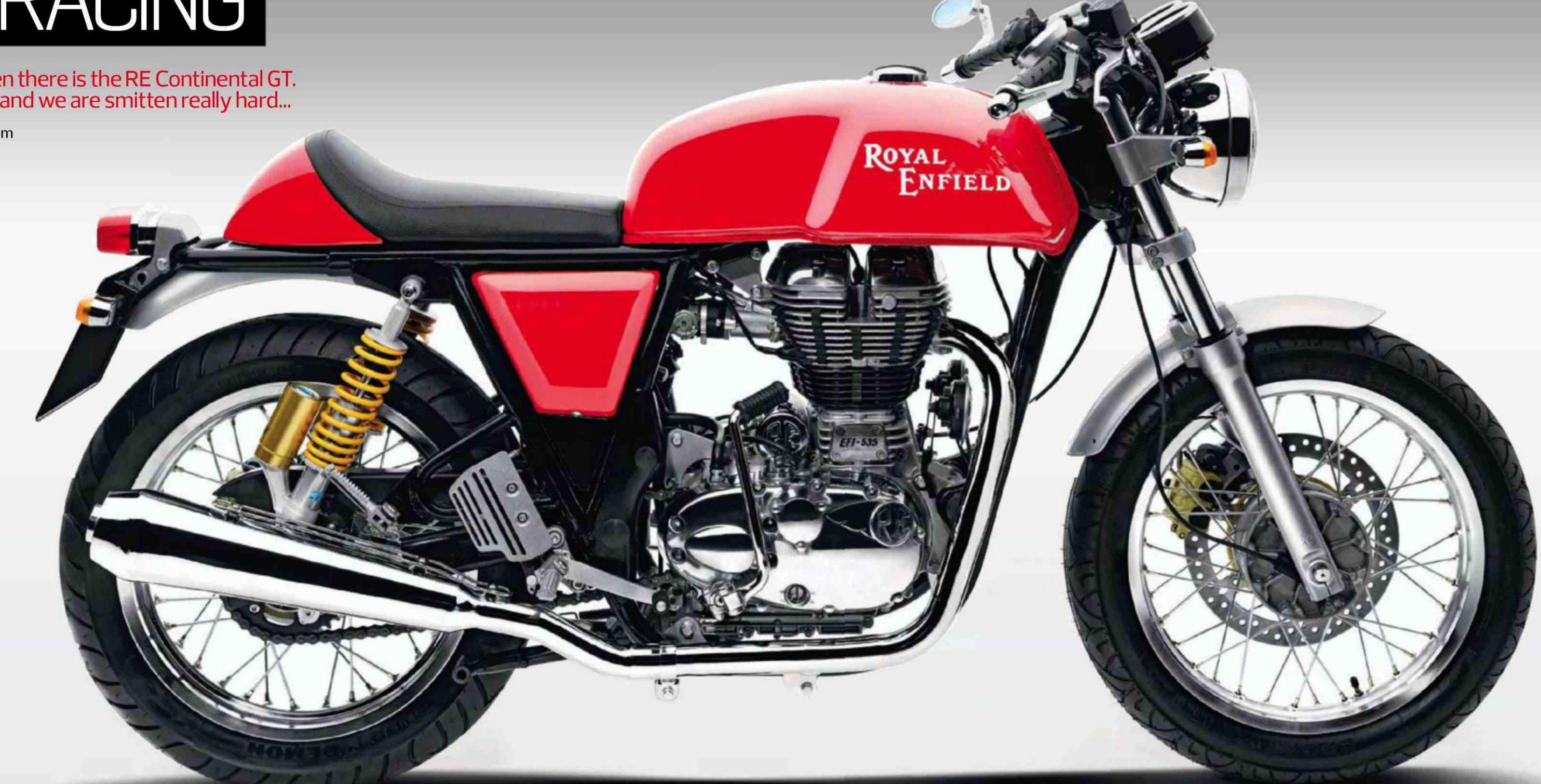
1 Power The RE Conti GT is the lightest and fastest RE now, but it is not as fast as the other bikes on the road. The engine is a massive 535cc powerhouse but is tuned to produce an output of just 29.1bhp @5100rpm and 44nm of torque @ 4000rpm. Go elsewhere if you want absolute bang for your buck.
